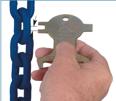
Inspection of material diameter
