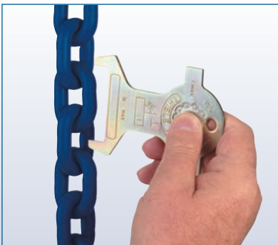
Inspection of permanent elongation
