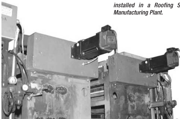
Specifically designed ultra quick Posidyne Clutch/Brake with flywheel and welded tubular base completely assembled.
